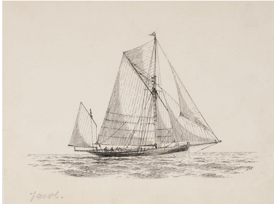
Figure 5.5. A drawing of a yawl-rigged vessel, similar to the Lilly Elena . A yawl differs from a ketch in that the mizzen mast is behind the steering mechanism and sticks out over the stern, whereas on a ketch the mast is forward of the steering.
