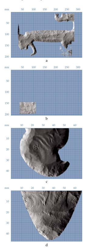
enough to capture key surface details (Figure B.2c). The lens setup with a smaller field of view would lead to much more detailed scans with as little as 0.06 mm between the measurement points (Figure B.2d).
