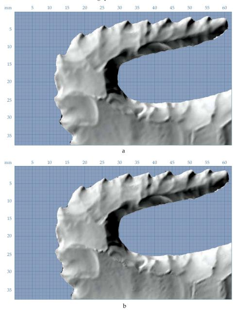
**Figure B.4.** Reliability threshold during scan merger: (a) close-up of a 3D model with high reliability threshold; (b) close-up of a 3D model with low reliability threshold (CPN-P-2707 / Artifact 90-12).
