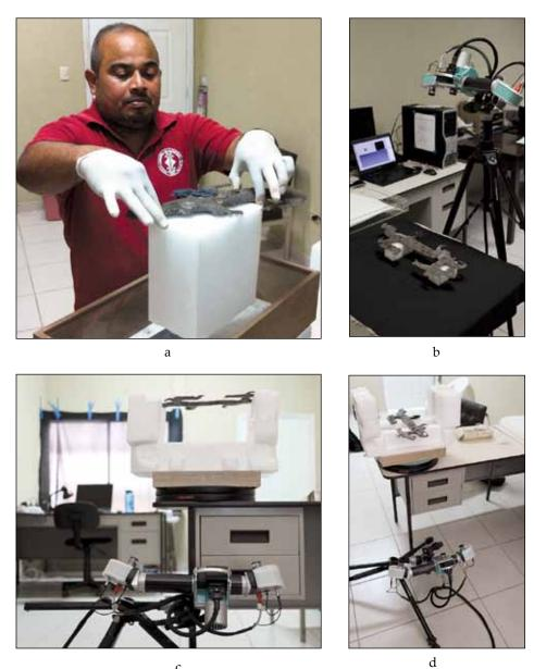
**Figure B.1.** Scanning procedure: (a) museum curator placing the artifact on a Styrofoam support; (b) scanning the top side of the artifact; (c) scanning the middle section of the bottom side; (d) scanning the tip of the bottom side.
